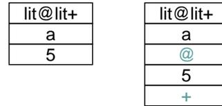
Figure 3: Threaded code for the superinstruction for a @ 5 + without and with slots for the optimized-away primitives
