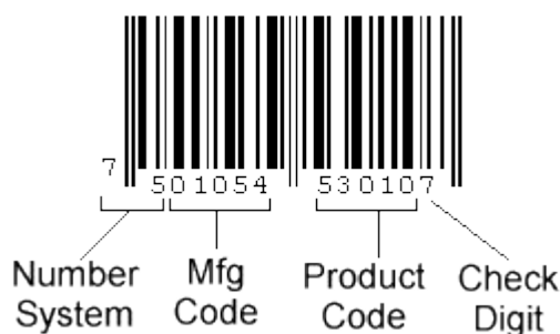
Fig. 3. The structure of data represented by EAN13 bar code
