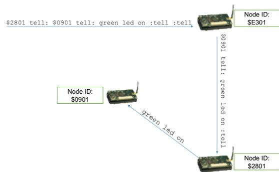
Fig. 3: Recursive employment of the `tell:` primitive. Once the node with ID E301 encounters the first `tell:` it parses all the following symbols until the last `:tell` and a frame containing `0901 tell: green led on :tell` is sent to node with ID 2801. The payload interpretation of the payload on the receiving side leads to the sending of a new frame destined to node 0901 with `green led on` as payload. Once received, node 0901 turn its green LED on.
