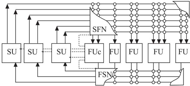
**Functional units (FUs)** aimed for data processing, external access and control operations. The number of FUs, destination, number of inputs ( $FU_i$ ) and outputs ( $FU_o$ ) can have wide range. Adding of inputs and outputs can extend the functionality of unit. It is necessary to found a compromise between complicated multifunctional FUs and simple single-functional units. It is obligatory the control device ( $FU_c$ ) in any processor.
